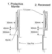
When building a recess the flueing must be considered. Shown right is the minimum distances possible when offsetting the flue to allow for a recess above.
